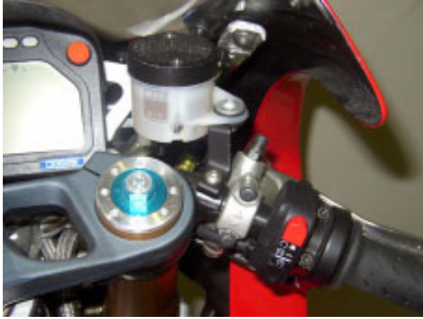
The front brake fluid reservoir is located near the front brake lever mount.
