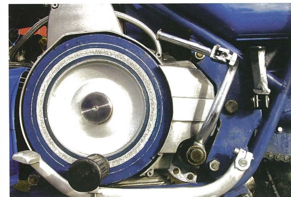
Left-foot kickstart, mighty brake pedal and that fearsome outside flywheel
